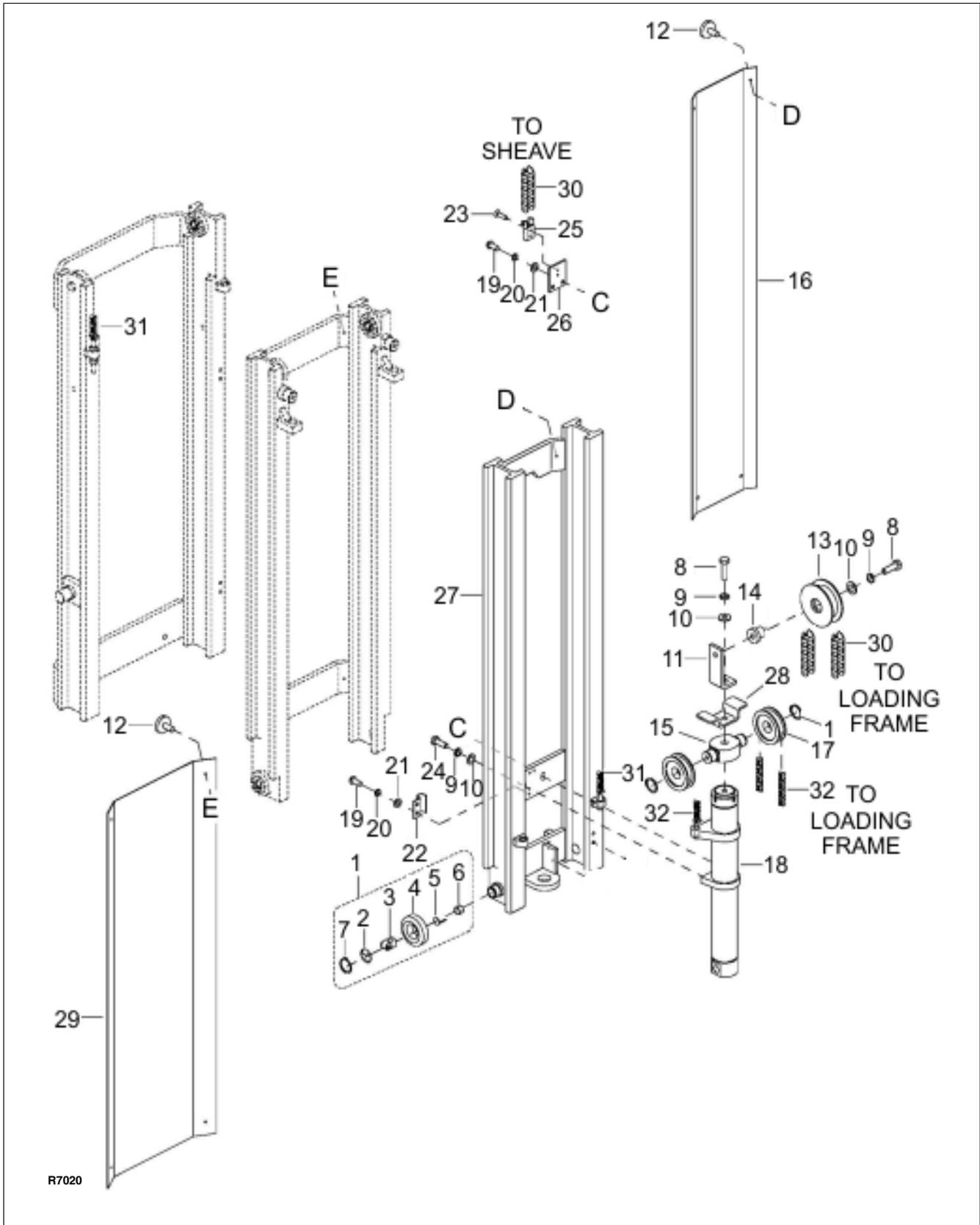
Figure 11-16 Elevation System (TRIMAST - Part 2)
