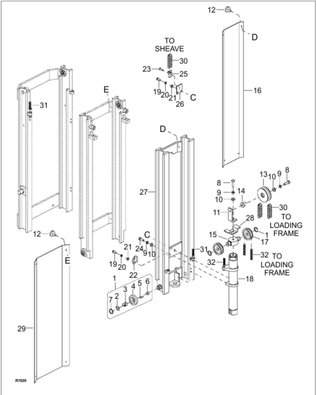
Figure 9-5 Elevation System (TRIMAST - Part 2)
