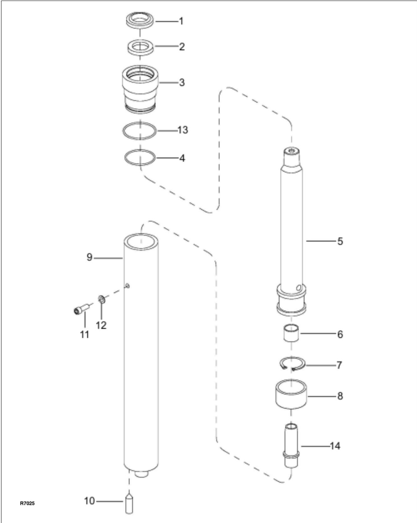
Figure 11-21 Lift Cylinder, Secondary (TRIMAST)
