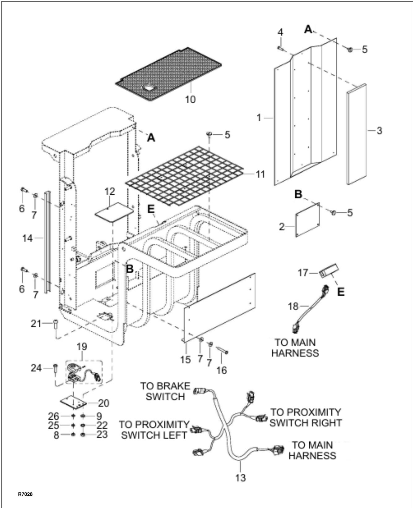
Figure 11-24 Loading Frame Assembly
