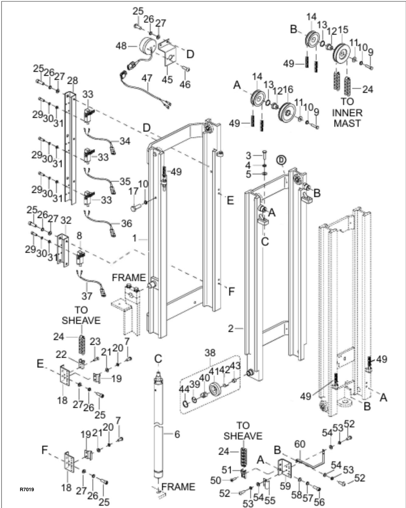
Figure 8-7 Elevation System (TRIMAST - Part 1)
