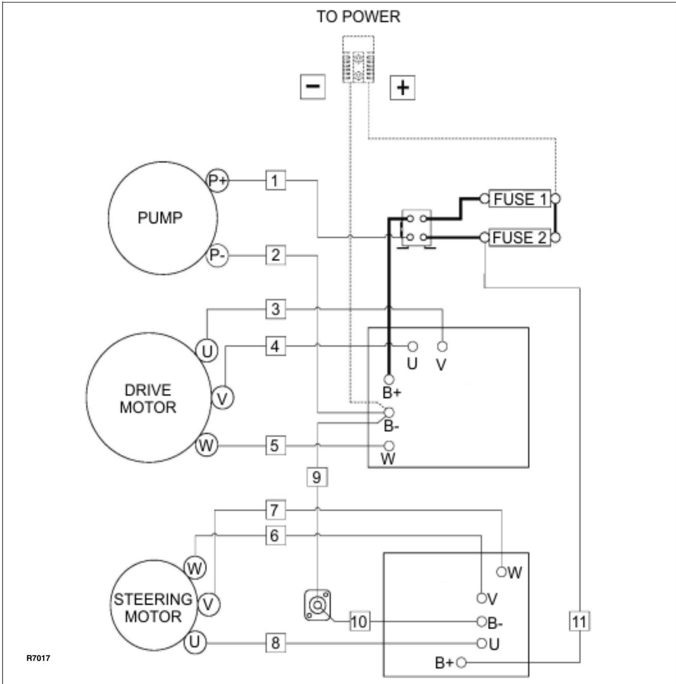
**Figure 11-13 Wiring Cables**
