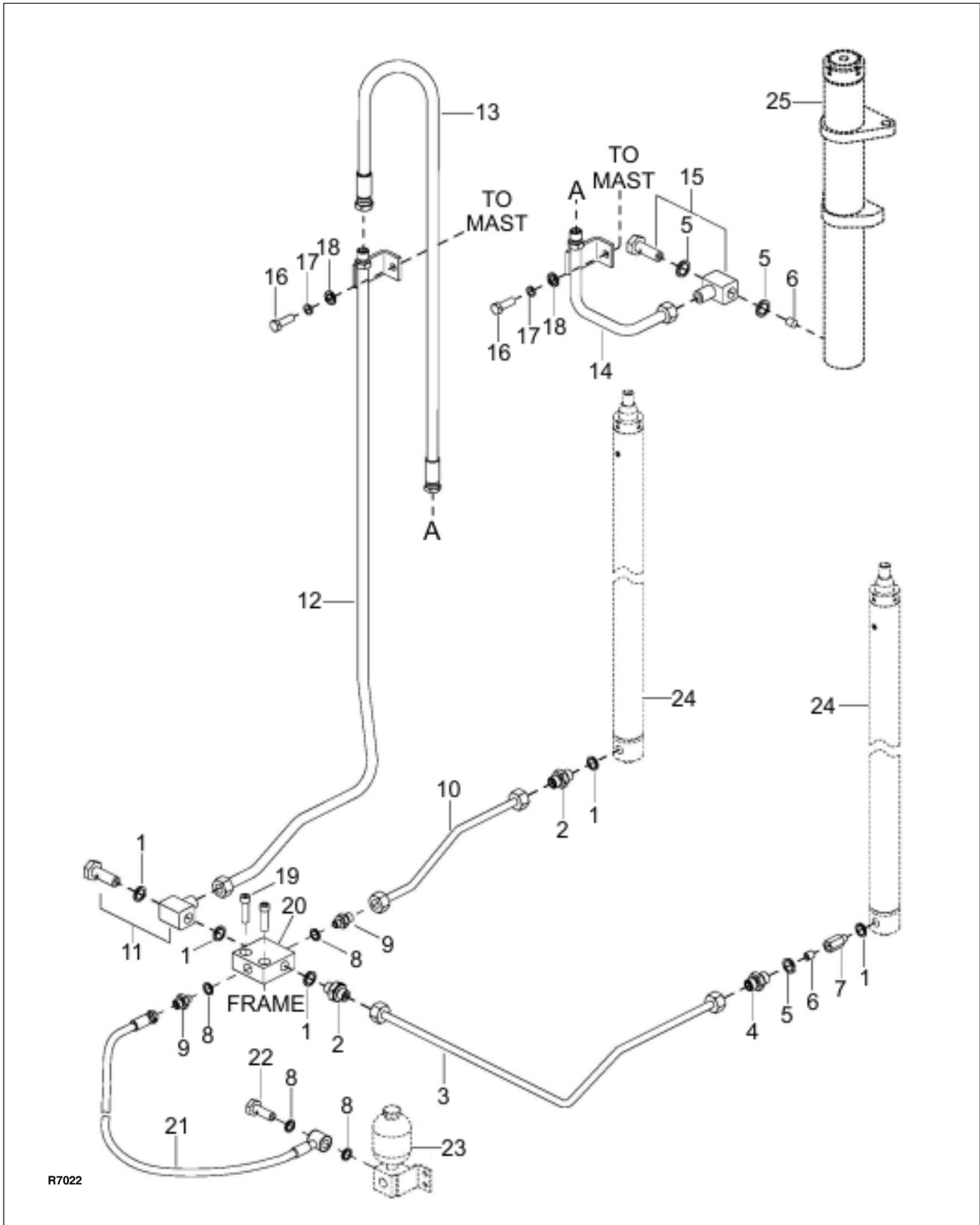
Figure 11-18 Hydraulic Lift (TRIMAST)
