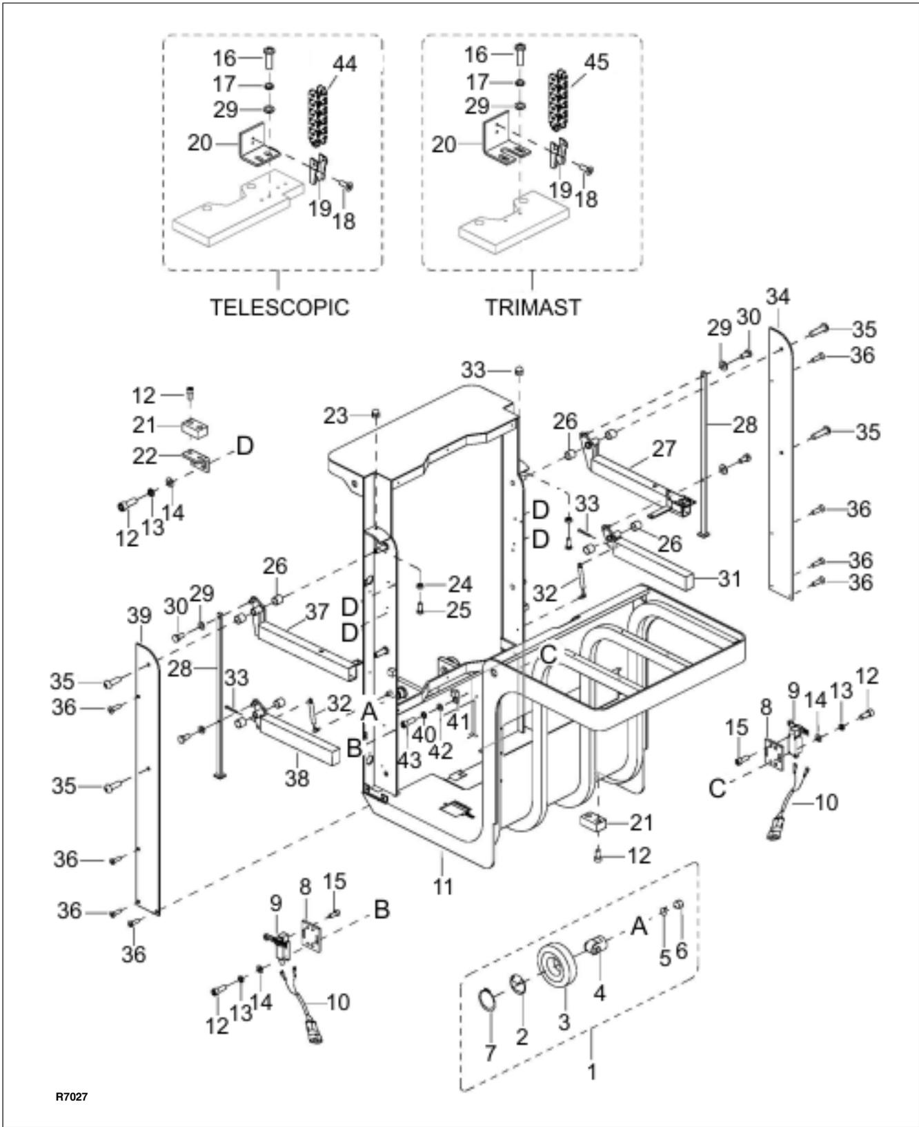
Figure 9-6 Loading Frame Installation
