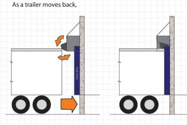
the Rain Deflector swings up providing a seal to the top of the trailer
