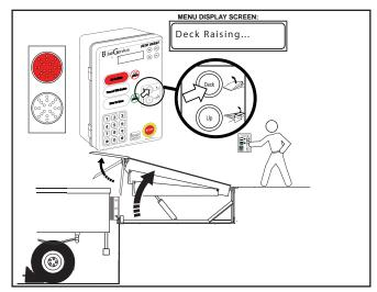
3. Release the 'Deck' button. The dock leveler will then descend with the deployed lip on the vehicle load bed and the LCD message will change to 'Deck Moving'. The outside traffic light remains RED (optional) and the control station light will turn GREEN (optional). Wait for the dock to fully deploy on the vehicle load bed before commencing loading / unloading operations. NOTE: Ensure that the full width of the lip overlaps the vehicle load bed by a minimum of 4" (102mm).
