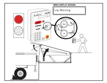
3. Once the lip has deployed, release the 'Lip' button. Both dock leveler and extended lip will descend onto the vehicle load bed. The LCD message will change to 'Deck Moving'. The outside traffic light (optional) remains RED and the control station light (optional) turns GREEN, advising dock staff that loading / unloading operations may begin. NOTE: Ensure that the full width of the lip overlaps the vehicle load bed by a minimum of 4" (102mm).
