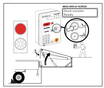
2. When the lip has fully retracted, release the 'Deck' button. The dock will fall back to the stored position with the lip resting in the lip keepers. The control station light (optional) will change from GREEN to RED, alerting dock staff that the transport vehicle is no longer available, and the outside traffic light (optional) turns GREEN, advising the truck driver that it is safe to depart.
