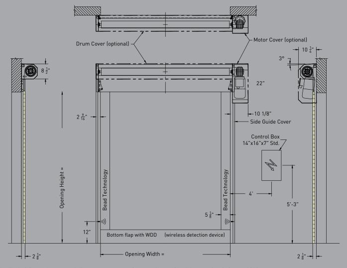
All indicated dimensions are net; the space necessary for mounting and maintenance has to be provided REMARK, based on the risk analysis of the environment, extra push buttons, detectors and covers might
