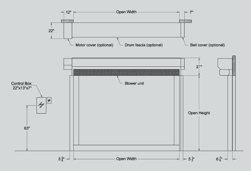
All indicated dimensions are net: the space necessary for mounting and maintenance has to be provided. REMARK: based on the risk analysis of the environment, extra push buttons, detectors and covers might be required.
