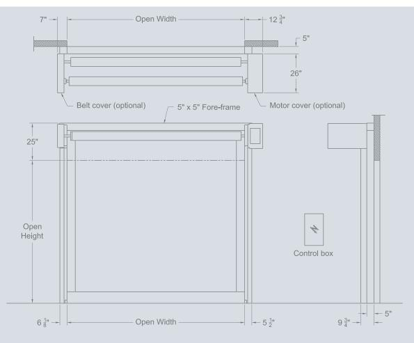
All indicated dimensions are net: the space necessary for mounting and maintenance has to be provided. REMARK: based on the risk analysis of the environment, extra push buttons, detectors and covers might be required.
