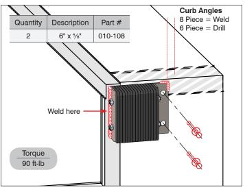
DB411WB welded to curb angle and installed with wedge anchors or embedded anchor bolts on six or eight piece curb angle.
