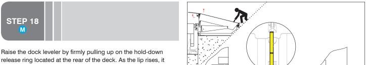
release ring located at the rear of the deck. As the lip rises, it will automatically swing up and extend. Let go of the release ring once the deck reaches full height. Engage the dock strut by following the instructions in Section 7.0 and walk down the deck until it is resting on the dock strut.
