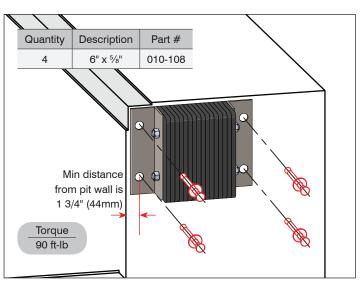
DB411 installed with wedge anchors or embedded anchor bolts on four piece curb angle.
