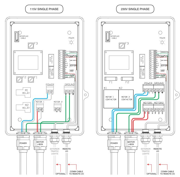
Blue Genius<sup>™</sup> control panel wiring layout for 115V single phase only.
