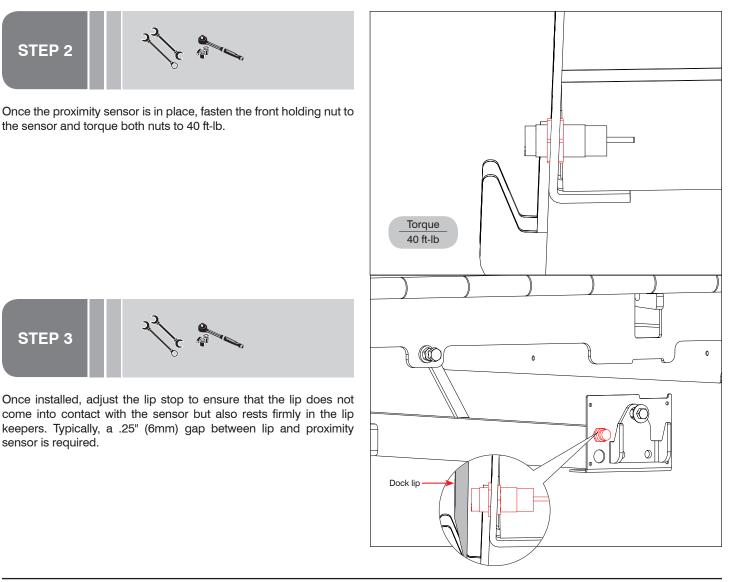
**STEP 3** Once installed, adjust the lip stop to ensure that the lip does not come into contact with the sensor but also rests firmly in the lip
