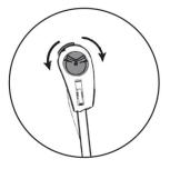
3. Turn the travel switch to move the vehicle forward or backward.
