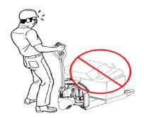
When leaving truck neutralize travel control. Fully lower lifting mechanism and set brake. When leaving truck unattended also shut off power.
