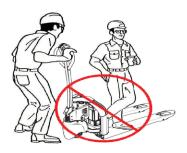
Observe applicable traffic regulations. Yield right-of-way to pedestrians. Slow down and sound horn at cross aisles and wherever vision is obstructed.
