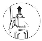
1.Lift the battery out of the vehicle.
