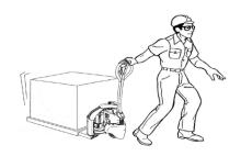
Use special care when operating on ramps; travel slowly, and do not angle or turn. Travel with lifting mechanism downhill.
