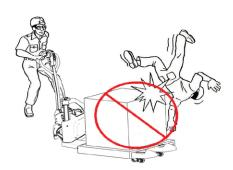
Start, stop, travel, steer and brake smoothly. Slow down for turns and on uneven or slippery surfaces that could cause truck to slide or overturn. Use special care when traveling without load as the risk of overturn may be greater.
