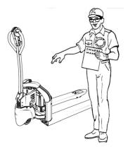
Do not operate this truck until you have checked its condition. Give special attention to wheels, horn, battery, controller, lift systems, brakes, steering mechanism, guards and safety devices. If you have any questions, notify your supervisor or proper authority.
