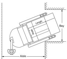
Note: Aisle dimensions listed above assume the minimum bay width to be straddle OD plus 5" (2.5" on each either side of straddle leg). Straddle OD is the load width plus 10". Truck performance may vary due to application requirements and chances in model design.
